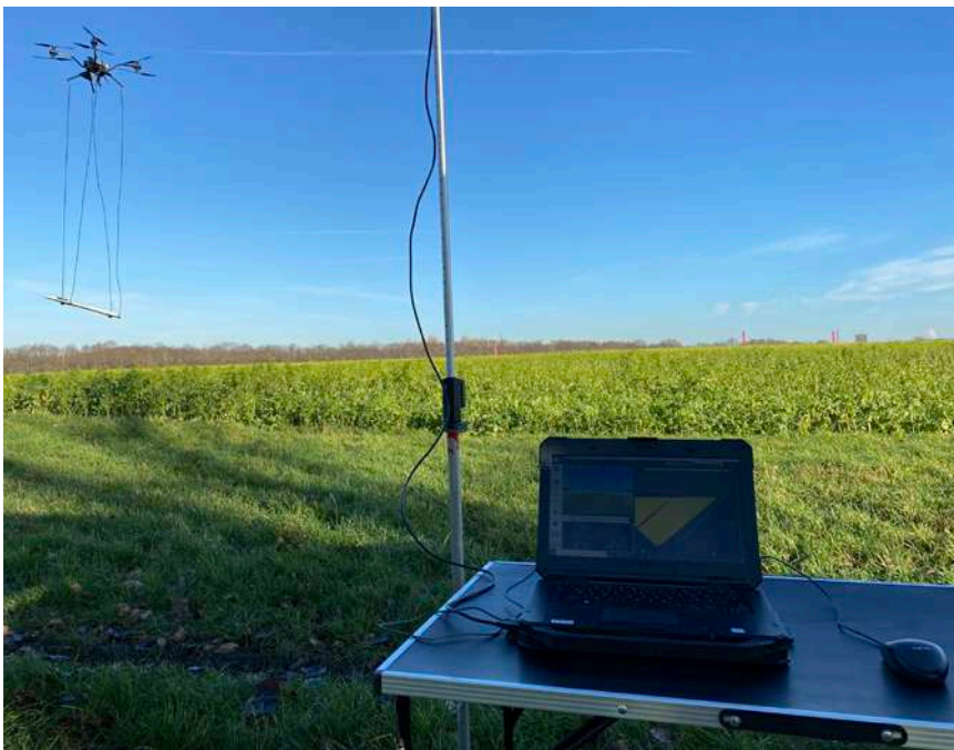
The drone geomagnetics system also flies over tilled fields and is about 10 x faster than conventional methods.
