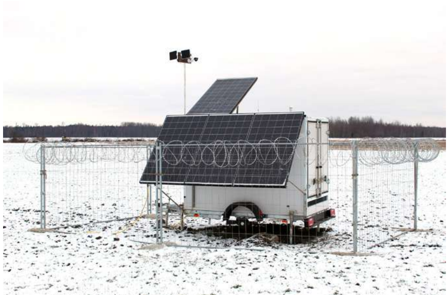
Wind measurement with Lidar and uSens designed trailer
