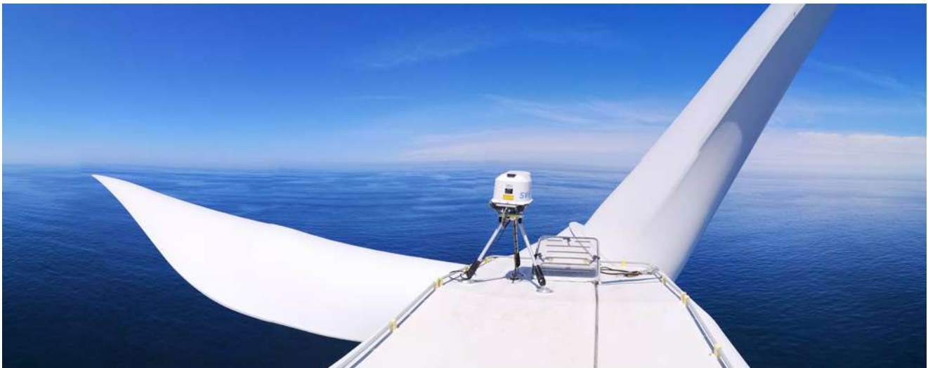
Photo of a wind lidar system on a floating wind turbine. As part of the VAMOS project, the influence of motions on the power curve was analyzed and corrected in real time. Photo: SWE, Universität Stuttgart
