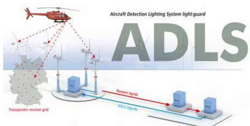
Functionality of the light:guard system for demand-controlled night identification
