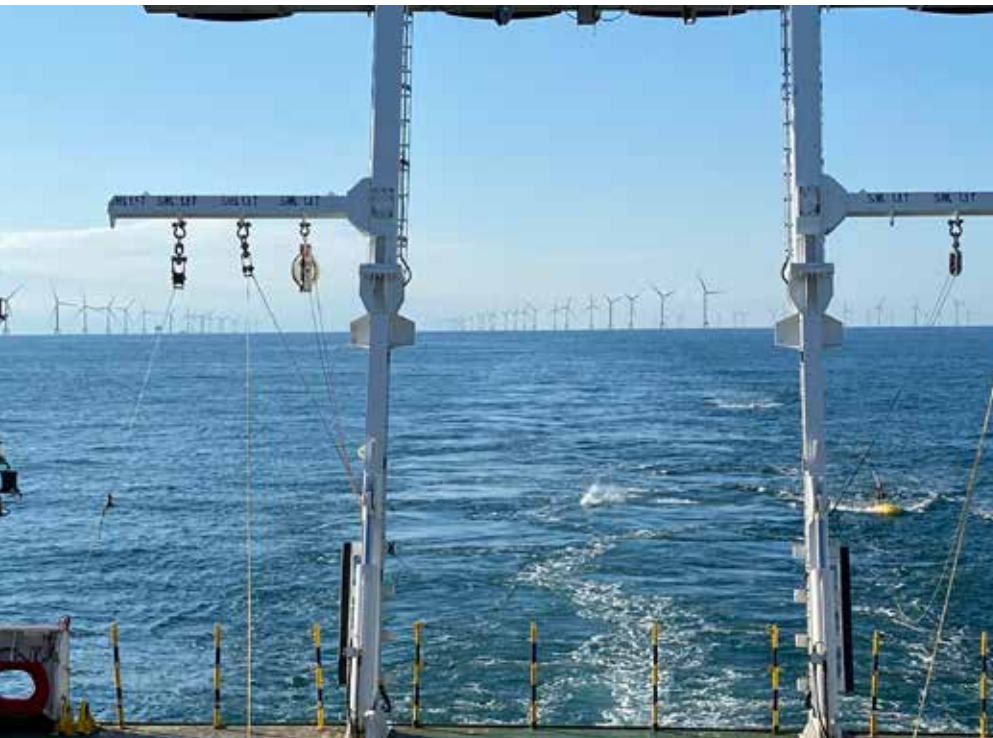
Fugro Pioneer running lines with seismic equipment deployed to perform a geophysical survey. ©Fugro
