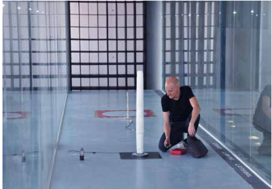
Testing the wind generator in a wind tunnel. Photo: Vortex Bladeless
