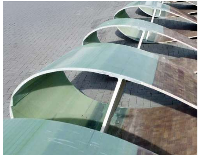
Rotor blade "filets", cut into smaller pieces, provide further insights into material properties. Photo: Fraunhofer IWES
