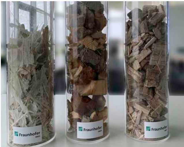
Separated rotor blade fractions: GFRP, PVC foam, balsa wood (from left to right). Photo: Fraunhofer IWES
