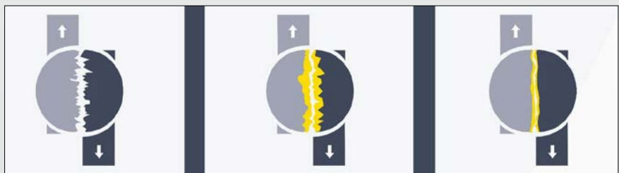
3 REWITEC surface modification steps.
