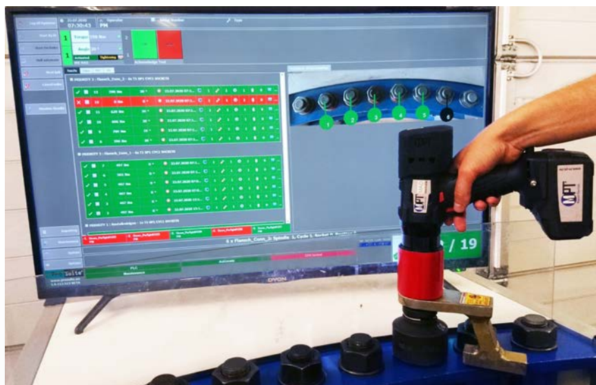
Bolting in the worker guidance system ProTight™ with battery torque wrench MAD 20.
