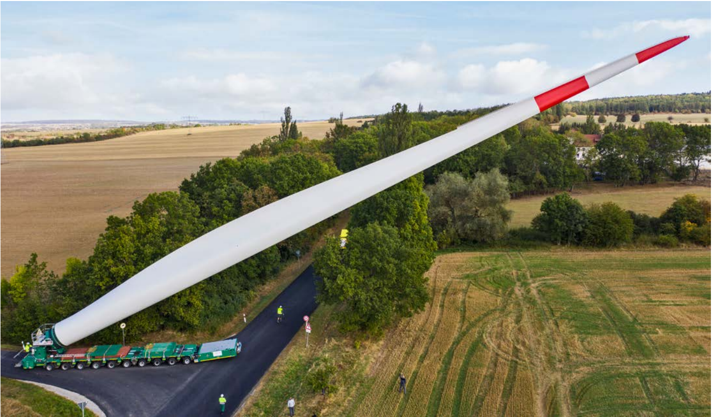
Transporting a 73.3 m long rotor blade for a Vestas V150-4.2 MW to Keula wind farm in Thuringia. Photo: Jan Oelker
