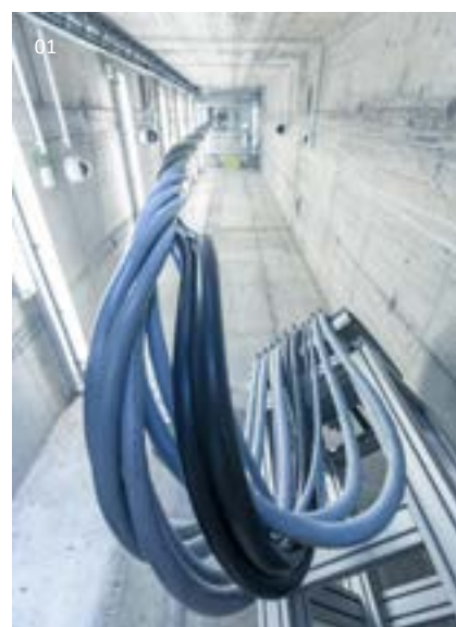
01 | In LAPP's unique test facility cables up to 12 metres in length are tested under realistic conditions
