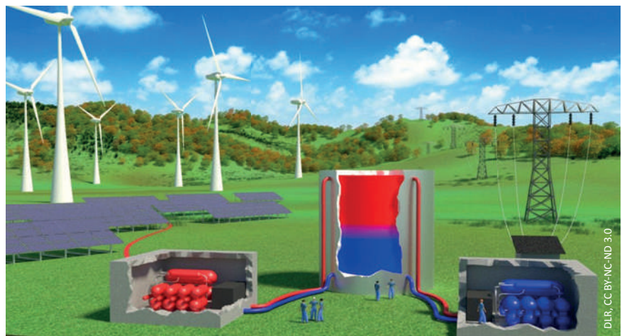
Carnot batteries are able to store electrical energy in the form of heat.
